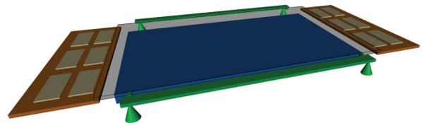
Figure 1: The tactile stimulator and the LCD screen (in blue). Force sensors (green cones) are used to measure the position of the fingertip.
