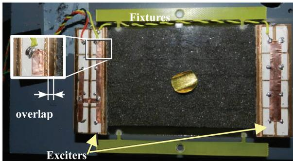
Figure 6: The manufactured tactile plate and its exciters during measurements; the yellow sticker is used for deflection measurement with a laser interferometer.
