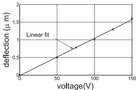
Figure 7: Deflection of the tactile plate for several voltage amplitudes (peak values). Experimental values (crosses) compared to a linear fit.
