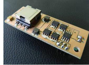
Figure 11: The electronic board of the DC/AC converter.
