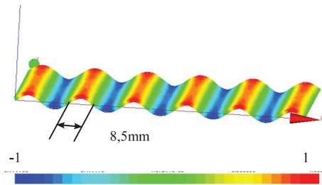
Figure 3: Simulation result of the deflection at 31,2kHz (arbitrary color scale).
