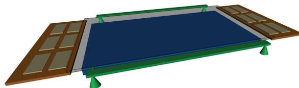
Figure 1: The tactile stimulator and the LCD screen (in blue). Force sensors (green cones) are used to measure the position of the fingertip.
