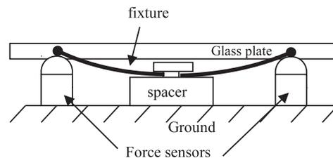
Figure 9: Mechanical arrangement of the force sensors. The frame is bent in order to preload the sensors (not to scale).
