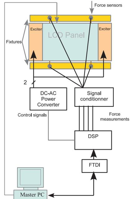
Figure 12: Connections between each component.
