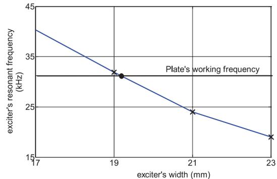
Figure 4: Criterion for exciter's width choice.
