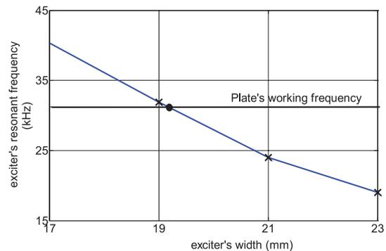
Figure 4: Criterion for exciter's width choice.
