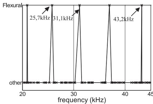
Figure 2: Vibration modes of the 93mmx65mmx0.9mm glass plate. Each cross represents an existing vibration mode.
