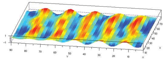
Figure 8: Measured cartography of deflection of the tactile plate; the exciters' vibration is not measured.
