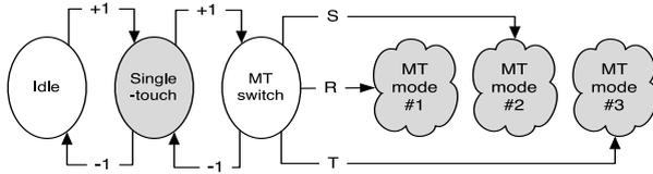
**Fig. 3.** Simplified view of a multi-touch state machine based on an RST classifier. +1 and -1 transitions are triggered by contact addition and removal. The R, S and T transitions are triggered based on the first principal transformation detected. Note that once in mode #1, #2 or #3, multi-touch interaction does not have to be restricted to the transformation initially detected.
