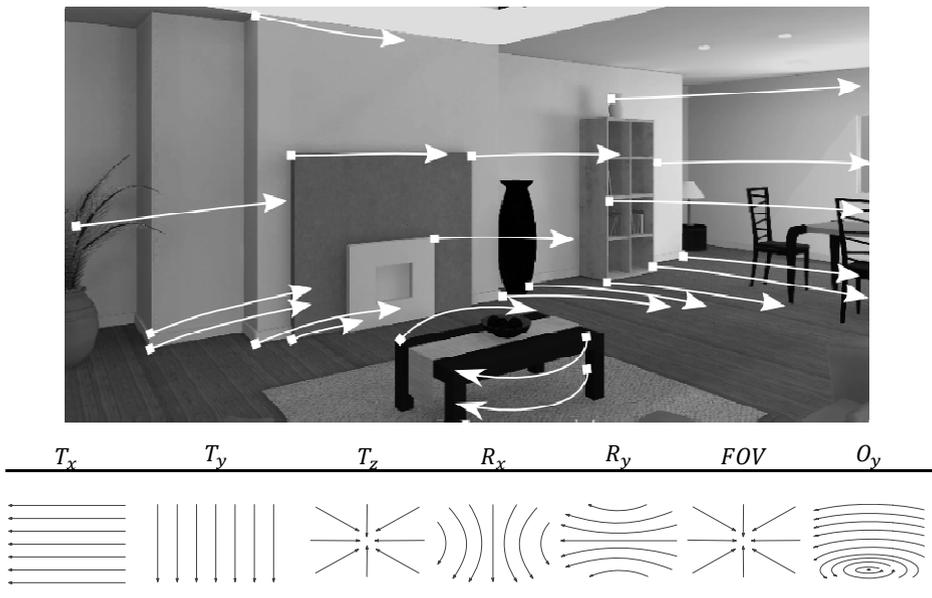
**Fig. 4.** Top image: optical flow computed over time with OpenCV when circling the viewpoint along the vertical axis ( $R_y$ ). Bottom images: stylized renderings of the flows corresponding to the 7 viewpoint controls of Table 2 (arrows could all point in the opposite direction).
