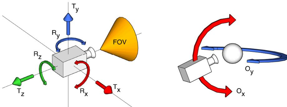
**Fig. 1.** Typical viewpoint controls: dolly, sidestep and fly ( $T_z$ ,  $T_x$  and  $T_y$ ), tilt, pan and roll ( $R_x$ ,  $R_y$  and  $R_z$ ), zoom ( $FOV$ ) and orbit ( $O_x$  and  $O_y$ )
