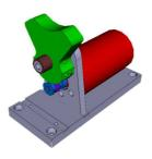
**Fig. 3.** A lever actuated by a DC motor through cable transmission. Iron brush bearings reduce friction.
